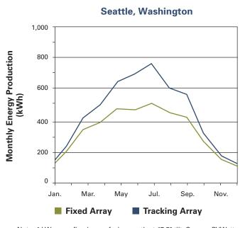
Note: 4 kW array; fixed array facing south at 32.1° tilt. Source: PVWatts
