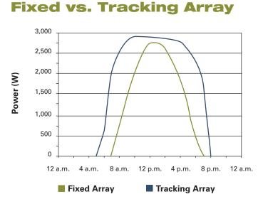
Note: 4 kW array; fixed array facing south at 32.1° tilt. Source: PVWatts. Daily power values calculated for average insolation values for May 19.
