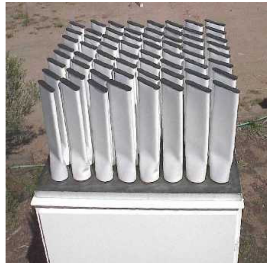
Prototype Quill Cool Cell with Flattened Radiators above the Lid
