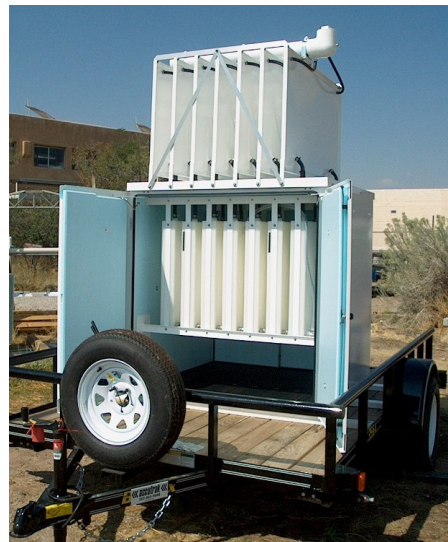
Trailer Mounted High Flux Cool Cell for Joshua Tree National Park Interior Showing Tanks, Radiators and Equipment Space
