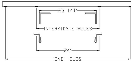
6. Finally space the J-Clips at a distance of **Measurement C**. Follow these steps for each P.V. module. After modules have been aligned, secure rail assemblies to the Track Rack™.
