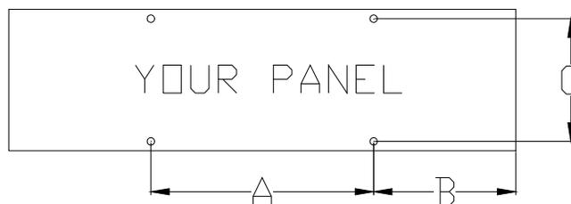
2. Now measure the distance from the edge of the P.V. Module to the edge of the panel. This is **Measurement B**.
