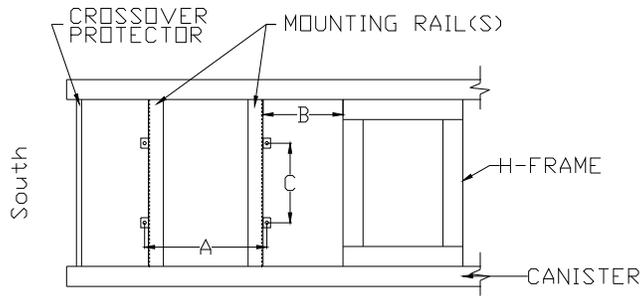
3. Take one mounting rail and place it on the H-Frame/Canister assembly at the minimum of **measurement B** with the down flange of the rail facing the H-Frame.
