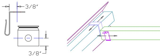
5. Subtract a distance of  $3/4'' \times 2 \times 3/8''$  to **Measurement A**. For our example this will produce a new measurement of  $23 \frac{1}{4}''$  or  $3/8'' - 24 - 3/8''$ .
